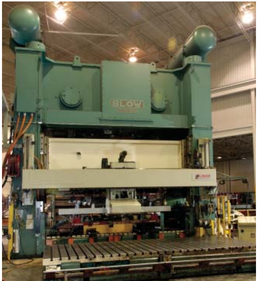
Egar Tool & Die outfitted this 1200-ton press with a front- and rear-mounted transfer system, enabling the company to win a multitude of automotive transfer jobs.
