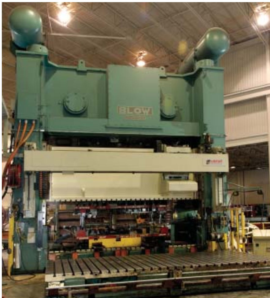
The transfer system can be shifted up and out of the way, allowing Egar to switch quickly from automated part transfer to progressive- or hand-transfer-die work.
