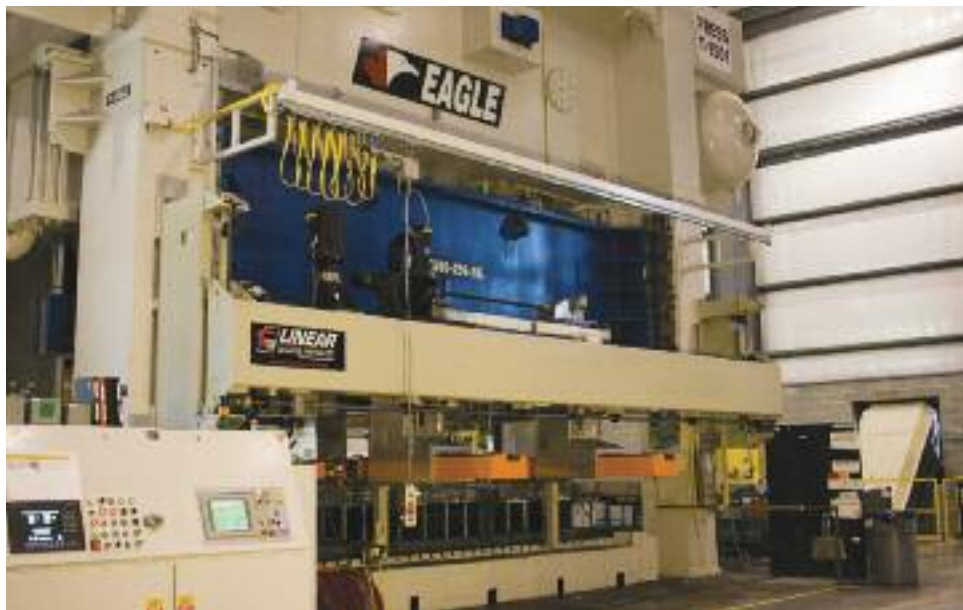
The front- and rear-mounted transfer system shown here is mounted on a 1500-ton mechanical press, with 256 by 96-in. bed, at Metrican Stamping, Dickson, TN.
