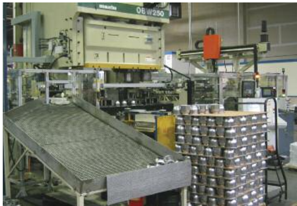
A servo-transfer system mounted on this 250-ton gap-frame press automates stamping of deep-drawn components.
