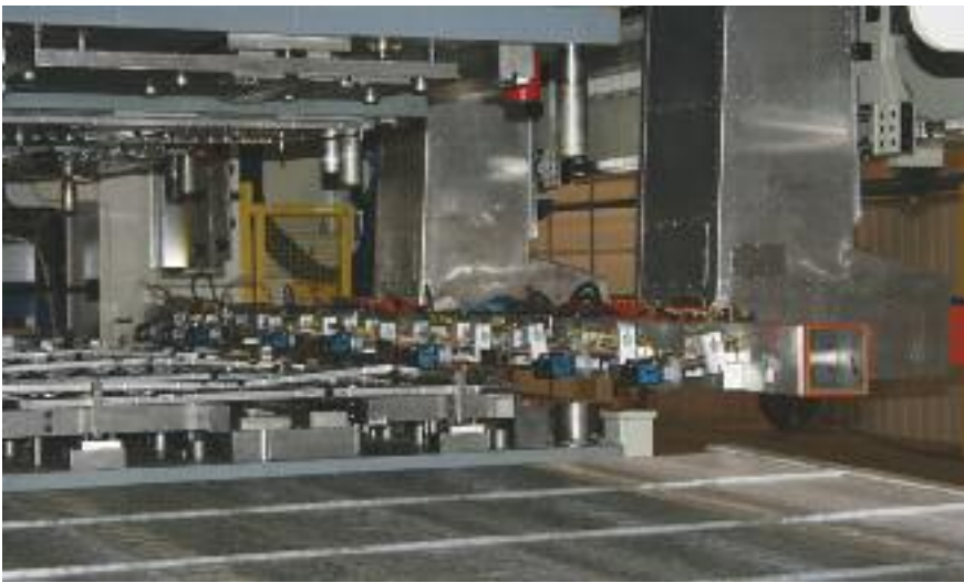
A common method for mounting end-of-arm tooling is use of a common plate located on the bars—which includes several fixed finger stations—shown here mounted on the inside face of the transfer rail of a front- and rear-mounted transfer system.
